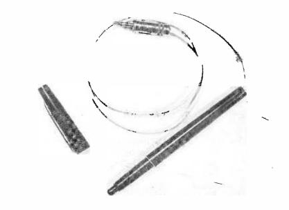
Photo 4: This shows a pen based on the TI type L-63 photocell, built using a marking pen case.
