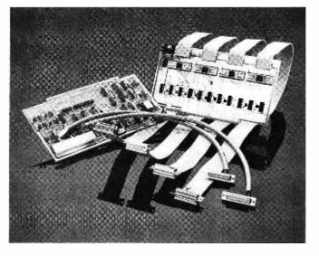
Two new ALTAIR 8800 I/O boards are now in production. These include a serial interface (88-25IO) that can be ordered with one or two ports, and a parallel interface (88-PIO) that can be ordered with up to four ports.
