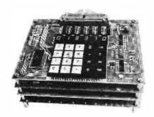
Here they are! The modular micros from Martin Research. The keyboard programs the computer, and the bright, fullydecoded digits display data and memory addresses. A Monitor program in a PROM makes program entry easy. And, even the smallest system comes with enough RAM memory to get started!
