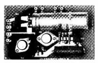
The assembled power supply card shown above powers the JOLT<sup>®</sup> CPU, I/O, and RAM Memory cards.
