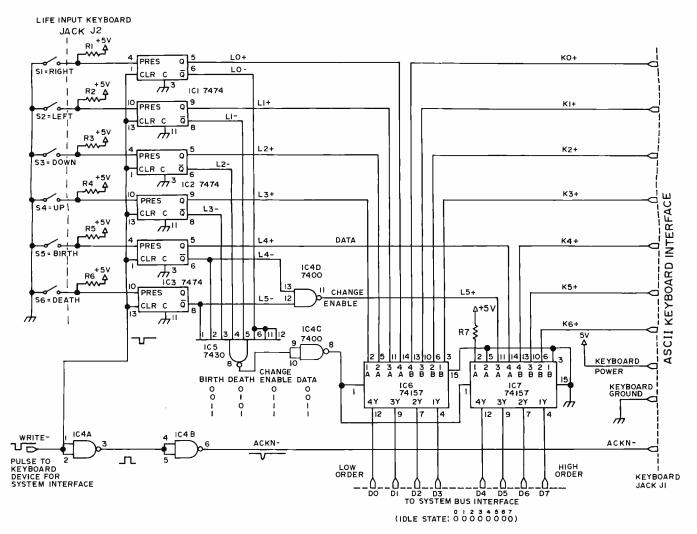
Figure 2: The logic diagram of a keyboard interface which implements the formats of figure 1. Resistors R1 to R7 are TTL pull up resistors. The value are not critical, and may range from 1 K0 to 10 K0, ¼ W.
