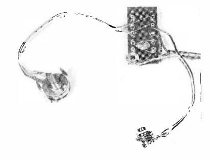
Photo 6: This photo illustrates how the circuit of figure 1 can be assembled using a small turret terminal board. The transistors and R5 are mounted out of sight on the rear side of the board.
