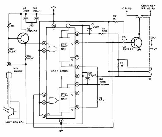
Figure 3: By adding a pair of oneshots to the circuit, the ability to draw pictures is improved through a short data lockout period which avoids smearing.
