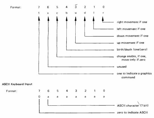
Figure 1: Data formats for graphic control commands and ASCII keyboard input.
