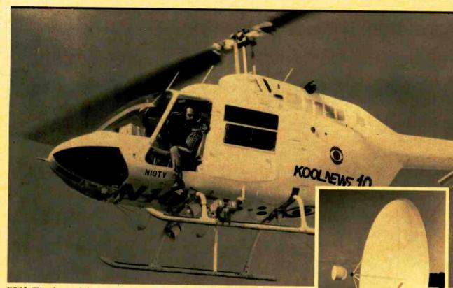
KOOL-TV makes two helicopter flights every day, including a live weather report. One of the helicopter's features is a retractable microwave antenna mount.
