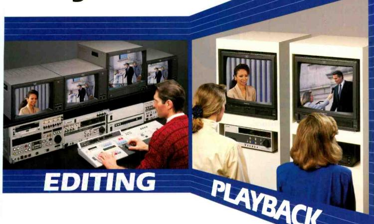
and postproduction applications. Like a luminance bandwidth of 4.5MHz, a K factor of 2% and a signal-to-noise ratio in excess of 50dB. It provides images that equal one inch VTRs with signal integrity that exceeds five generations of recording.
