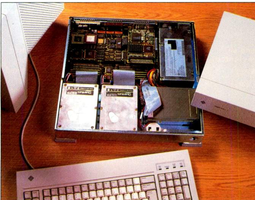
Internal view of SPARCstation 1.
