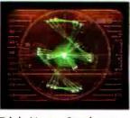
Triple Vector Overlay– SMPTE Bars on A, B and C inputs delayed by 6° and 12° to demonstrate phase error
