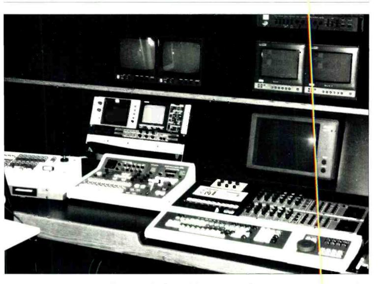
Basic test equipment—a Magni WFM560 waveform monitor and Tektronix 1420 NTSC vectorscope—is integrated into Edit Room 1 at Frame Runner in New York City.
