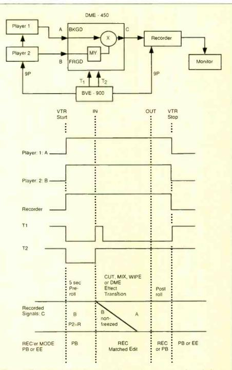
Figure 3. Typical system interconnect and timing chart for two-machine playback editing.
