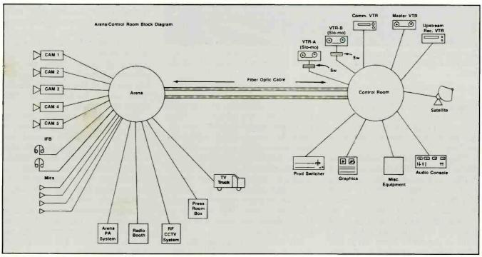
Figure 2: Full arena-to-control room block diagram.
