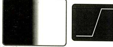
**Figure 2**: To create wipe patterns in a switcher, a waveform generator produces the control signal. Here a simple vertical split screen with soft edge is created by providing a ramp with a short risetime. Edge softness is adjusted by increasing or decreasing the risetime of the ramp signal. For a soft-bordered wipe, two ramps, offset in time, would create transitions from A to matte and from matte to B.
