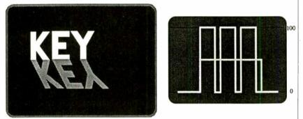
**Figure 5:** By precisely setting the black level of the external key signal to 0 and the white level to 100, the external key can take over control of the video mixer. Black in the key signal becomes the background and white becomes the foreground. Control signal levels in-between become a mix of background and foreground. The intermediate portion of the key above will be a mix of background and key video: the key video could be black creating a shadow, or a color causing a glowing effect.
