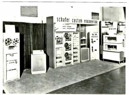
The original Schafer Automation System, the Model 60, known as the "blue wire job," on display at the 1959 NAB convention. Concert One reel-to-reel decks were wired to two Seeburg juke boxes that played 45 rpm records. Also, the first spotter machine, with an Ampex deck, which ran re-wind and fast forward to locate commercials. Schafer: "It took at least 100 clip leads to make it work at the convention."
