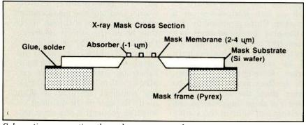
Schematic cross-section through an x-ray mask.
