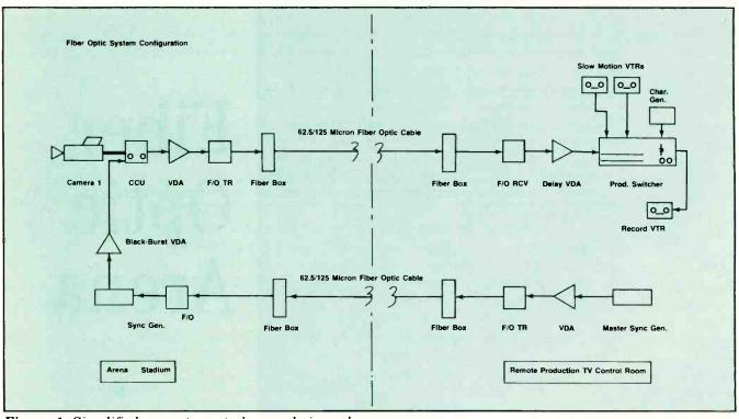
Figure 1: Simplified arena-to-control room design scheme.
