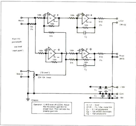
Figure 2: Active, line-level M-S matrix (unbalanced)
