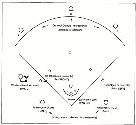
Figure 1: A proposed stereo baseball microphone layout.
