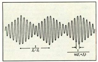
**Figure 1**: Waveform with beats due to pure tones with frequences  $f_1$  and  $f_2 = f_1 + df$ .
