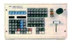
special effects. The all-solidstate VSR-10 uses VLSI chips to give you 34 seconds of memory and maintain original image quality.
