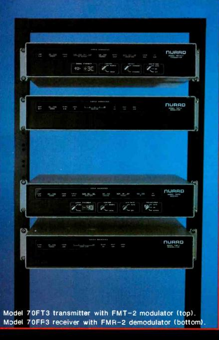
For STL/ICR and other point-to-point microwave applications, Nurad offers the state-of-the-art in transmitters and receivers. The 3-Series of microwave equipment is a family of integrated IF heterodyne transmitters and receivers that can be configured for any desired system application.
