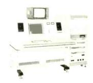
The Asaca/Shibasoku ADR-5000 is a magneto-optical video disk recorder that inputs signals in digital form.
