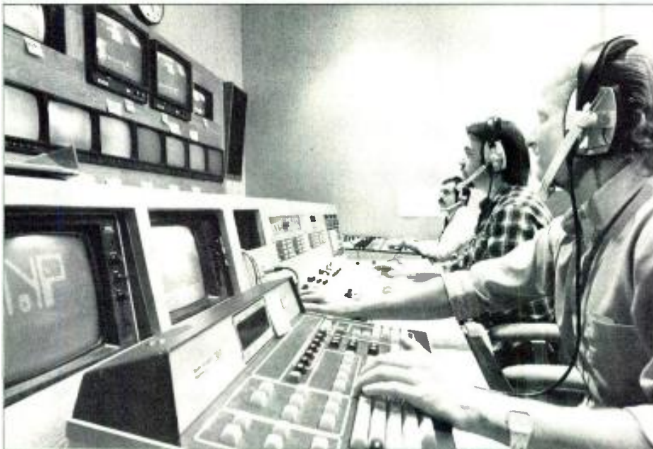
Within KIMO-TV's production control room, David Bellamy (left), graphics operator; Mike Southern (center), technical director; and Jerry Floyd, senior post producer, prepare for an evening news broadcast. Bellamy is operating a 3M D-8800 electronic graphics keyboard, while Southern operates a switcher made by The Grass Valley Group, Inc. Floyd is in charge of an ADM 1600 II audio board.
