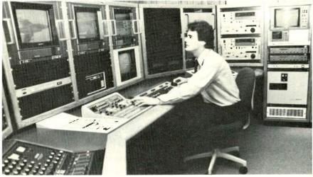
ISC Technologies' new computerized editing suite features the Paltex Editstar computerized editor, Hitachi HR-230 one-inch, two Sony BVU 800s, Chyron RGU-2, Harris HDE-100 digital effects unit, and Yamaha's M512 audio mixer.
