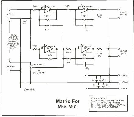
Another flexibility lies in the fact that the M and S outputs can be recorded directly, without going through the matrix. Then the stereo can be produced in post-production, allowing the operator to set the stereo width and the perspective to match the need at each point in the program.
