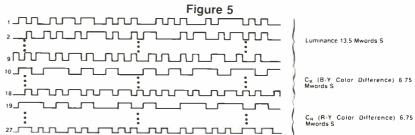
Figure 5 results from digitizing the signals from Figure 2 and sending them down eight pairs for each signal—a total of 24 pairs carrying signal data. Each group includes a ninth pair for a reference and timing signal. All 24 bits are sent in parallel, while words representing sample locations are sent serially through the 27 total pairs. The data rates are 13.5 Mwords/s for the luminance group and 6.75 Mwords/s for each color difference group.
