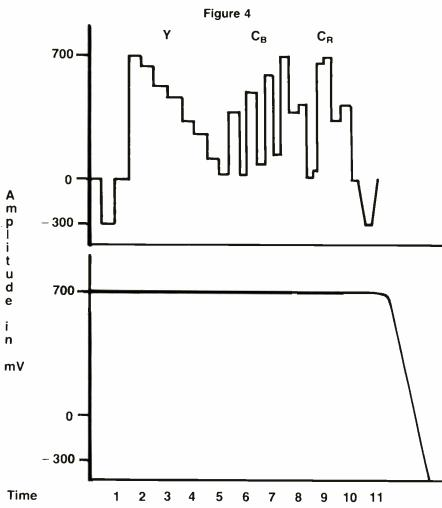
Figure 4. Waveform and spectrum for the time division multiplex (TDM) form of analog components, S-MAC. It consists of Y compressed 2:1,  $C_B$  compressed 4:1, and  $C_R$  compressed 4:1. The  $C_B$  and  $C_R$  portions of the waveforms are derived from  $P_B$  and  $P_R$  by offsetting their baselines to + 350 mV. The time compression yields a bandwidth of 11 MHz.
