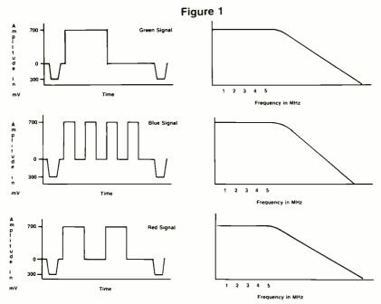
Figure 1. Color bars are shown on three channels to serve as a reference for examination of the various forms of component signals. Amplitudes are 700 mV for the video signals; 300 mV of sync is added for a total of 1 V. The spectrum of each signal is also shown. A baseband bandwidth of 5.5 MHz minimum is assumed. Interconnecting RGB signals over separate channels and circuits yields the most basic form of analog component interface.
