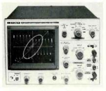
A stereoscope like that above can be used to check channels switched together before a stereo program is put on the air. A pattern like the oval seen indicates a phase difference that must be analyzed and corrected.
