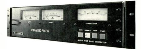
The Phase Fixer, a digital audio TBC, inserts a stereo pilot tone to correct time delays.
