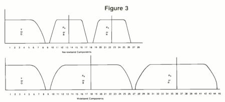
Figure 3. Spectra of frequency division multiplex (FDM) schemes in both narrowband and wideband forms. Luminance or green is carried in baseband. The other components are modulated on carriers. Amplitude modulation is shown because it minimizes bandwidth. Frequency modulation would yield better performance and would be preferable, but it would increase the bandwidth.
