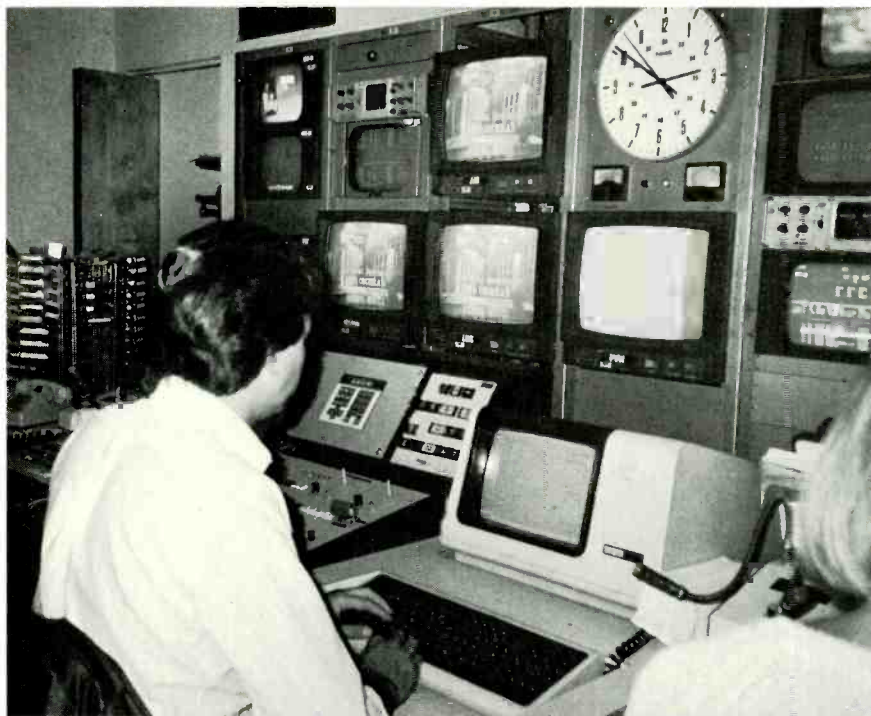
Vital's SAM system at WLS, the ABC O&O in Chicago, has turned an on-air local control room into the station's focal point as it rolls tape machines, runs commercial breaks and picks up the network.
