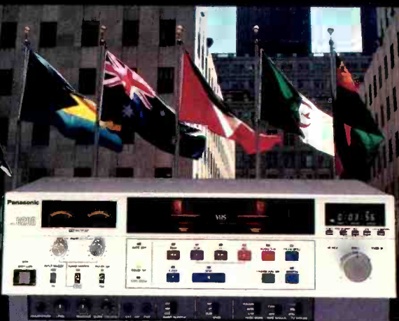
AG-6200E Multiformat VHS recorder for worldwide use: PAL, CCIR and 4.43 MHz NTSC. 14-step dial search.
