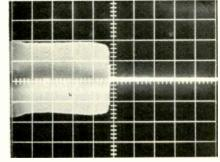
Fig. 3 Cue Output when machine stops. (Sweep = 10 ms./div.)
