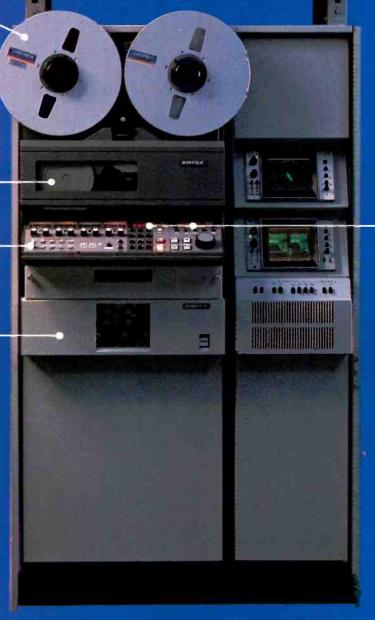
DUAL NUMERIC READOUTS— ONE FOR TAPE TIME/TIME CODE; ONE FOR CUE POINTS, DIAGNOSTIC CODES, TAPE SPEED, SETUP CODES
