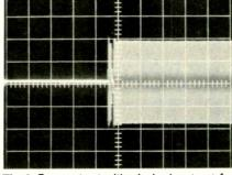
Fig.2 Cue output with air dashpot set for 105 ms. start delay (Sweep = 20 ms./div.) 90 ms. start delay (Sweep = 20 ms./div.)
