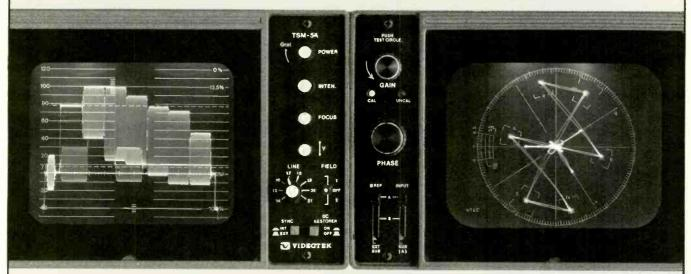
Line Select and 1H/2H Mode highlight the 1984 refinements to the ever-popular TSM-5A Waveform Monitor and VSM-5A Vectorscope. VIDEOTEK and service remains an uncompromised goal.
