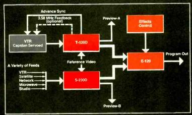
DT\* operation is possible with the T-120D with a single cable interface to the SONY\* BVU-820 U-MATIC\* VTR.
