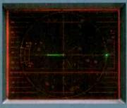
Dot placement on the +x axis indicates an error in the color frame matching of two signals.
