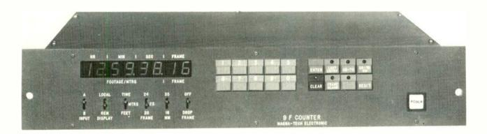
Frame rates of 24, 25 and 30 frames are selectable from the front panel with the 30 frame dropframe and non-dropframe selectable.
