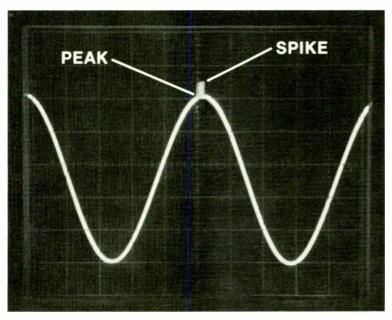
TFT's new FM/Stereo and SCA monitors make modulation uncertainty a thing of the past. Based on more than 14 years of experience with over 5,000 monitors, these new instruments have an exclusive (pat. pending) Peak Differentiator that separates true modulation peaks from the spikes generated by noise, overshoot and multipath distortion.
