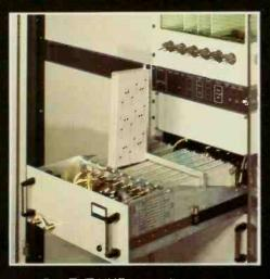
Pye TVT UHF transmitters cover peak sync powers from 10 to 110kW. All incorporate a highly sophisticated i.f. modulated drive system with solid state control logic for unattended operation and modern safety features. (You can, if desired, update the existing exciter of your current transmitter). All cover the whole UHF frequency range.
