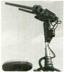
Linear actuator adjusts tilt of Nurad antenna.
