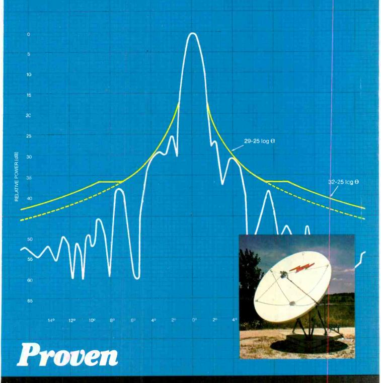
"Proven" means that the new Ancrew 4.5 metre receive-only earth station antenna has been thoroughly evaluated on our automated test range. Far-field range testing provides essential proof of antenna performance. As can be seen in the pattern range data shown above, 2° performance is available today. This 4.5 metre antenna will minimize adjacent satellite interference. It's 4 GHz patterns surpass FCC requirements—for 2° satellite spacing—enacted in August 1983.
