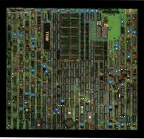
FORTEL's exclusive UNITEC single P.C. board construction (above) provides light-weight (less than 15 lbs.), low power consumption (less than 100 watts), and rugged-durability in a single rack unit (1¾-inch high); and all at a price that is thousands of dollars less than other manufacturer's TBC's. Exclusive "personality" program cards provide easy interchangeable use with any major brand of Type "C" 1-inch VTR or ¾" U-Matic.
