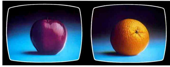
The apple (above left) was processed through a conventional TBC and shows quality loss including chroma noise, ringing, detail loss and luma/chroma timing error. The orange (above right) was processed through a Y-688<sup>32</sup> TEC and the result is a sharp, crisp, more life-like picture.
