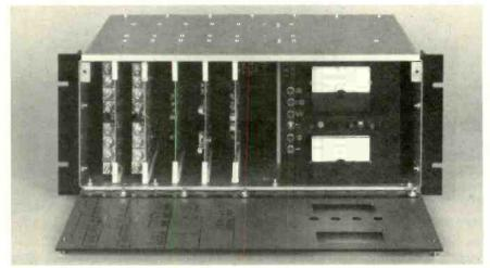
TFT's AM stereo exciter for C-Quam transmission.
