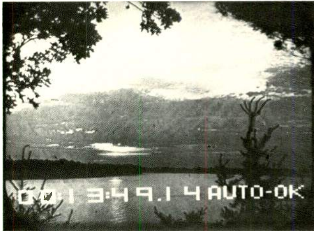
A character generator in the viewfinder of Harris's TC-90 ENG camera displays time code and auto setup status superimposed on the picture.
