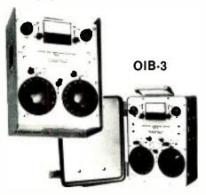
The Operating Impedance Bridge measures the impedance of networks, radiators, and the like while they operate under full power. VSWR as well as complex impedances of up to 400 ± j300 ohms can be
