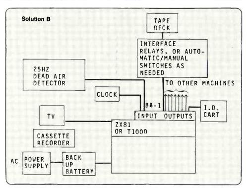
myself, mostly out of curiosity, Basic programming on a Sinclair ZX81. I purchased a BB-1 control module from Byte-Back Company (Leesville, SC) with eight independent S.P.S.T. relays and eight independent TTL inputs.
