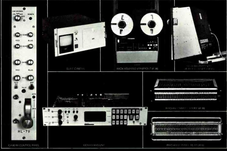
1. AFA JOY STICK CAMERA CONTROL PANEL (RCC-200 Series) Provides mobile and studio operations with a fast, simple method of controlling camera shadings.
