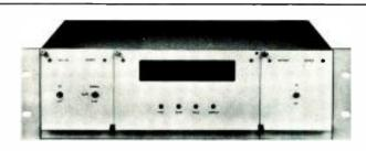
ESE Masters provide a means of keeping all time displays in the system in agreement, through the use of a Serial Time Code, Only one pair of wires is needed to distribute the time code to all ramota serial input displays
