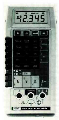
measurements for ac signals to 100 Hz, frequency to 200 kHz, and resistance measurements to 300 megohms. It also has the ability to store any measurement as a positive or negative relative reference value. Voltage is displayed in dBm, referenced to 600 ohms or in relative dB. Continuity testing, conductance, and constant current source diode testing functions are also included.
