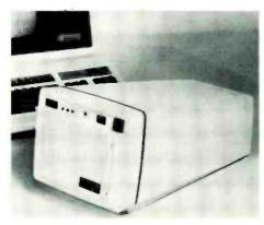
ics on film. It is a 35mm slide producing system which provides computer graphics users with the ability to quickly and automatically produce either a 35mm slide or an instant photographic print. It connects in the same loop as the CRT monitor by cables with standard BNC connectors.
