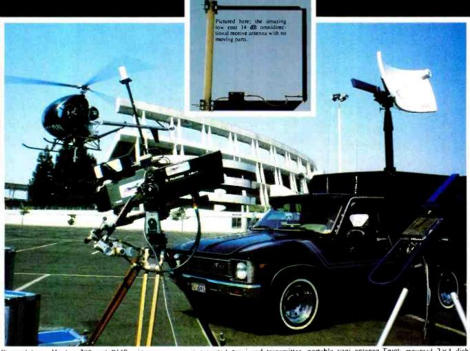
Pictured here: Hughes 300 and BMS microwave, camera mounted omni and transmitter, portable yagi antenna. Truck mounted 2×4 dish
