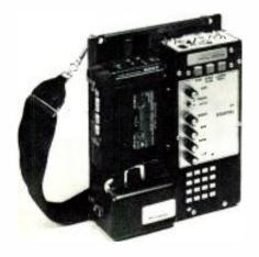
This field unit plugs into a telephone to feed back to a station with the reporter providing commentary over the recording. When equipped with earphone along with a microphone, full talkback capability is possible. A 16-button keypad can be ordered and, when used in conjunction with a dual tone generator, the Tele-File can supply remote control of station equipment.
