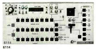
The 6114 is a broadcast quality, eight input, three bus video switcher. It features 12 patterns, positioner, event timer, pattern modulator, soft wipe, spot lite, blink key, toggle, take preview, automatic or manual mix and wipe blanking processor, nonsync lamp, loop through video inputs and a blackburst output. Price: \$4,680 PAL \$5,680
