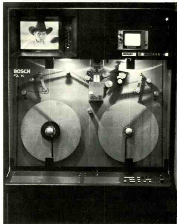
Transfers take place through the Fernseh FDL-60 film scanner which uses CCD imaging technology. Both positive and negative, 16-mm or 35-mm film can be accommodated
