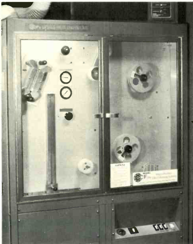
Before transfer, all negatives are carefully cleaned using the Lipsner-Smith CF-2000 system
