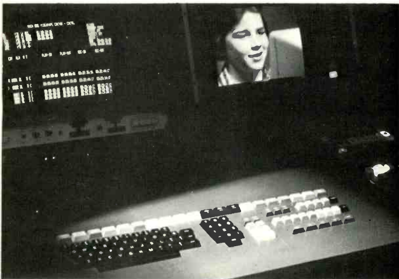
Workprint editing data is converted from feet and frames to timecode for videotape assembly using the Mach One editing system
