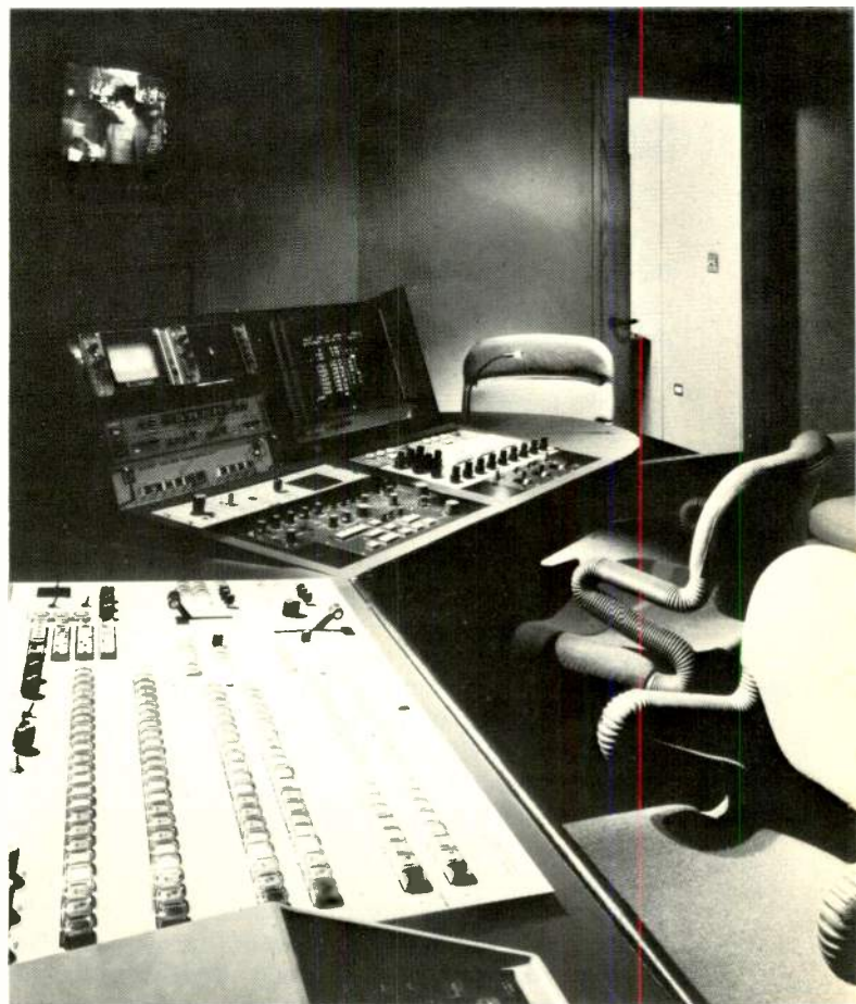
The color correction system is controlled from this room at Chicago's Editel
