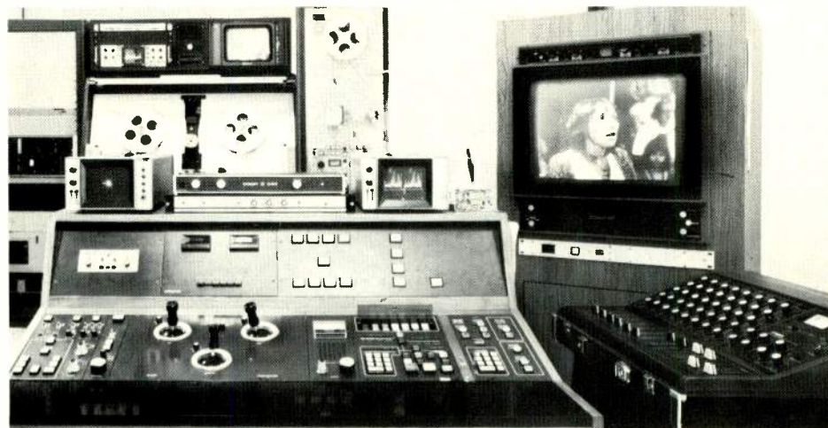
The initial transfer takes place in CFI's Rank Cintel Flying Spot Scanner room
