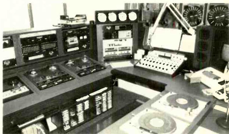
Overall view of studio, with turntables on right, tape machines left, automation system visible through window at rear
