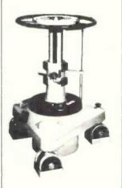
41 TERN PNEUMATIC PEDESTAL supplied with single litting steering ring, pedal-operated change over from crab to tricycle steering, adjustable cable quards, 7" dual duthane wheels. 20lb. total frim weights
