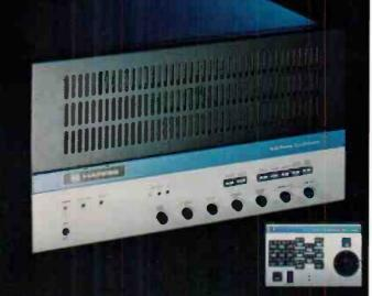
630 Frame Synchronizer: Component-coded framestore with TBC. Compressor/Positioner and Digital Noise Reducer optional.
