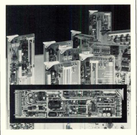
Introducing a GVGTM video distribution amplifier flexible enough to provide adjustable delay from 65nsec to 550nsec! Also; six outputs and optional cable equalization, all in ONE COMPACT PACKAGE,
