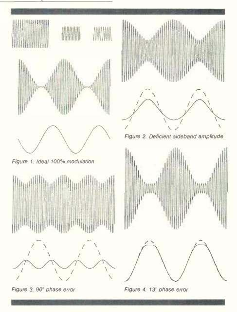
additive stereo system, the sidebands need not remain equal, but should be nearly conjugate: their magnitudes should be equal and their phases the negative of each other. The amplitude should be within 7 percent of equivalence and their phases should be within four degrees of conjugation.
