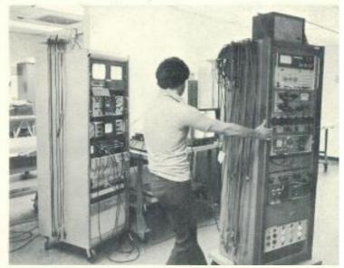
Test bays are mobile so that movement of disassembled gear is minimized
