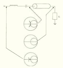
Figure 10. Series-resonance compensation
