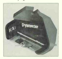
a head amp, according to the manufacturer. Recommended tracking force is 1.5 gm. The stylus is an elliptical diamond, and the unit also features super permalloy armature and tapered aluminum cantilever. The maker states that this cartridge is designed for exceptional musicality. \$126. DYNAVECTOR SYSTEMS USA.
