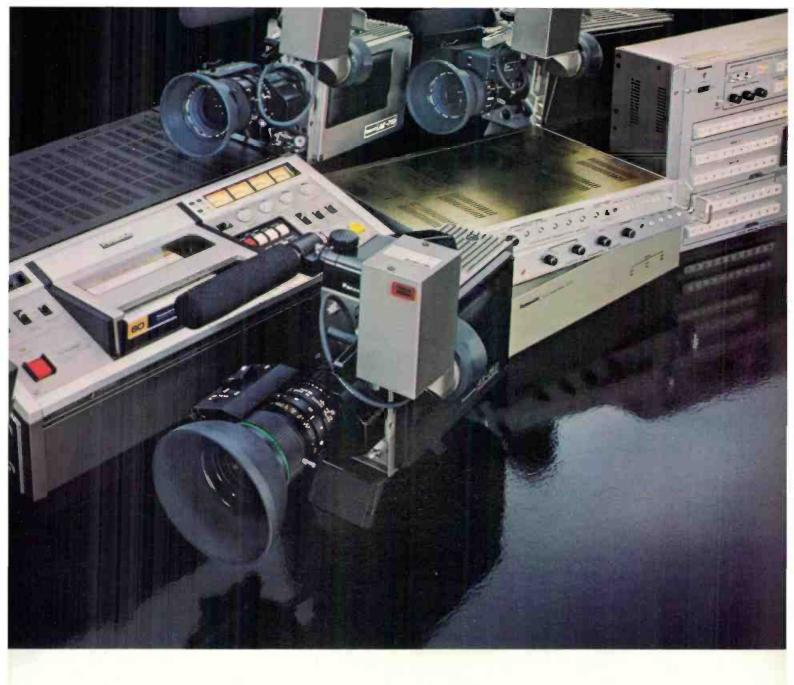
back beam control, the AK-760 has the necessary beam current to stabilize scene highlights to the point where comet tailing is greatly reduced.
