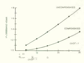
Figure 11. Limitations of series-resonance compensation
