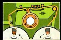
"PRO" tape path reduces dropouts
