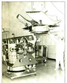
Engineers lower feedhorns and antennas onto RCA's newest commercial communications satellite
