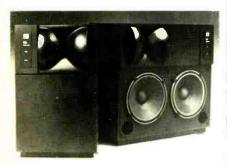
provides smooth, flat frequency response at all coverage angles on or off axis, according to the manufacturer, allowing great flexibility in speaker placement. The horn is coupled to a compression driver, crossed over at 1000 Hz. The speakers have 15-inch low-frequency drivers (one in the 4430 and two in the 4435). Maximum power output is 300 W for the 4430 and 375 W for the 4435, JBL
