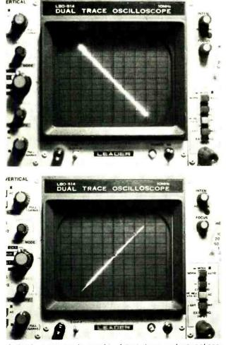
A simple scope can be used to detect stereo and monophase. Here, mono is shown out of phase (top)... And here it is in phase (bottom)
