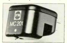
other MC cartridges. Specs include a 0.3 by two mil line contact solid diamond stylus, with a 0.16 mV rms at 5 cm/sec/1 kHz and 0.12 mV peak at 3.54 cm/sec/1 kHz output voltage. Coil impedance is 8 ohms ±1.3 ohms at 1 kHz, load impedance is 10 ohms or higher, and total cartridge weight is 7.5 gm ±0.3 gm. \$325. FIDELITY RESEARCH.
