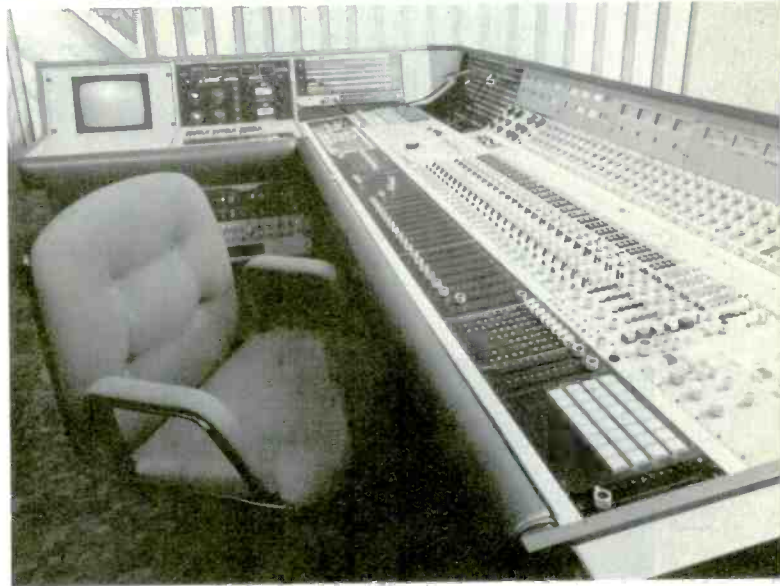
Audio console in the sweetening room has a recording console as its heart and is extensively supplemented with processing and synchronization equipment
