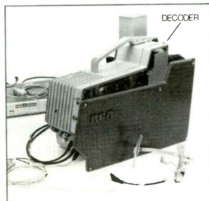
RCA TK-76B shown with decoder nearly "sandwiched" between camera body and door.
