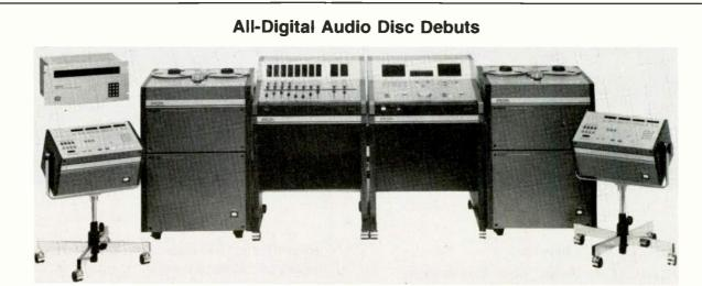
Matsushita's digital recording system consists of (left to right) delay/premonitoring unit, remote control unit, four-channel player/recorder, mixing unit, and editing controller
