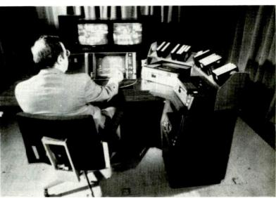
The CBS off-line electronic editing system. Now undergoing field trials, the system will make a major dent in the cost of electronic post-production for prime-time programs
