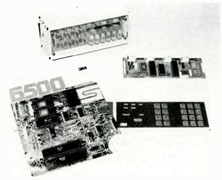
Some of the hardware for 3M's new 6500 microprocessor-based machine control system
