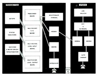
Block diagram of Telesis transmitter monitoring system. Sixty-four control channels operate external functions
