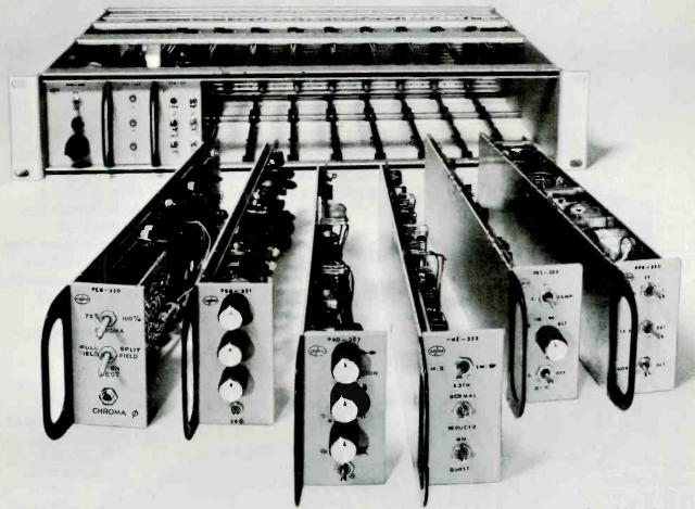
This totally integrated modular video test set is designed for the discriminating professional. The Lenco 300 System lets you specify video test signals to meet your system requirements, not the manufacturer's.
