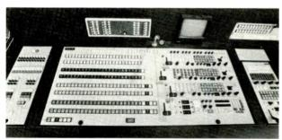
Control room console at Outlet Broadcasting's WJAR-TV. Vital 1600 switcher is the meta-controller
