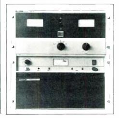
to drive two 50 W amplifiers, which in turn are coaxially combined by a hybrid combiner. A resistive reject load is used to absorb excess RF power if one of the final amplifiers should fail. The B-9100 also contains an internal harmonic filter. McMARTIN INDUSTRIES.
