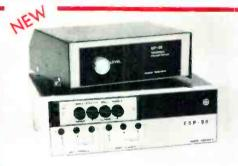
TURNTABLE PREAMPS. Leaders in their field. MP-8 & SP-8 — Bal. out; 0.05% dist.; 68dB gain; +8dBm out (+21dBm max); S/N —77dB down ref. to 12mv in @ 1kHz & +8dBm out. ±1dB RIAA, remote scratch & brilliance activation. Mono, stereo, table top, and rack mount versions. \$98 to \$162.
