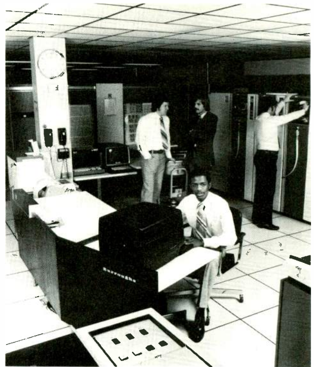
The other end of the spectrum in computer size and power is the two Tri-Processor Burrough's 6700s which can handle all the business and traffic affairs of the more than 180 radio and TV stations in the U.S. and Canada that are BIAS clients
