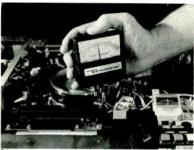
Shown measuring the critical supply tension on a Sony U-matic 2850.
