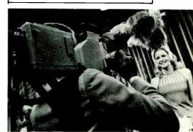
Microcam head and electronics pack on shoulder brace
