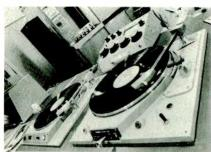
New Russco electronic-control turntable (left), mechanical-control table (right)
