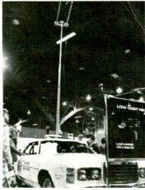
Telescoping mast is mounted on car roof
