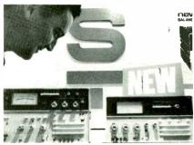
Sound Technology audio test source (right) and automatic distortion meter (left)
