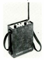
went into effect August 1, 1977. Model RPU-1103 has a rechargeable Nicad battery that runs the unit for eight to ten hours, at a 30% duty cycle. Unit has strap allowing easy operation on the
