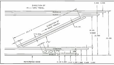
SMPTE Type C1-in. helical video recording format. Proposed record locations and nominal dimensions.
