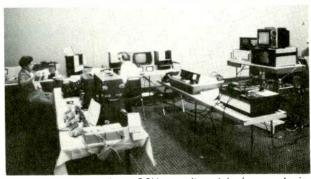
Portable switcher, editors, CCVs, monitors, telephones, etc. in on-location control room.
