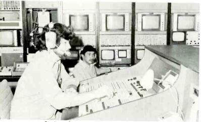
Studio and camera control at Prudential. John Kenlon, producer, is operating Grass Valley 163G switcher. Edward Reyer, systems engineer, is at CCU console.
