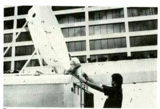
Program produced on location is beamed by satellite to other hospitals. Transmiter antenna (12 GHz) is beamed at experimental CTS satellite.
