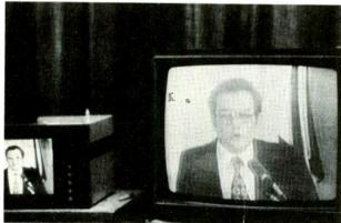
These monitors show signal before and after satellite transmission. The two-second delay can be disconcerting.
