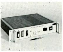
mote control over the range 3700 to 4200 MHz, for a frequency modulated video signal, with audio program subcarriers. It includes a down converter, phase lock demodulator, video processor, audio subcarrier demodulator, and associated power supplies. Frequency control circuits use COS/MOS logic, for high noise immunity with local or remote BCD control. HUGHES AIRCRAFT CO.
