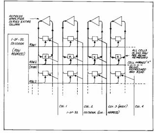
Fig. 14. System requiring only 32 refresh amplifier.
