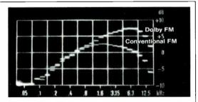
Real-time analysis of Dolby FM receiver output when tuned to interstation noise, using Altec Hewlett-Packard 8050A analyzer. In a "perfect" FM system the trace would be a continuously rising straight line. Thus the results show that highly modulated high-frequencies can be reproduced with significantly improved accuracy using Dolby FM.
