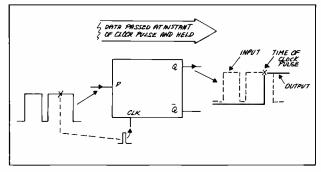
Fig. 3B. A flip-flop is clocked.
