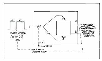
Fig. 3A. Flip-flop extended to remember data.
