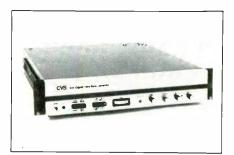
PAL is corrected composite video; for SECAM it is synchronized RGB that can be routed to an RGB switching system. The unit can also act as a PAL/SECAM converter with a plug-in SECAM option. Thus either PAL or SECAM in can be PAL or SECAM out. Unit has genlock signal generator; color dropout compensation; line by line velocity compensation; digital color averaging; a processing amplifier; and a 2-line window. CONSOLIDATED VIDEO SYSTEMS.
