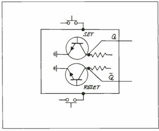
Fig. 2. Flip-flop with two outputs.
