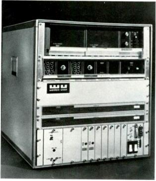
Typical of electronics in satellite systems which are helping bring the audio of the 80's is this control unit for Western Union receive-only radio earth terminal. Unit has capacity for six 15-kHz radio programs.
