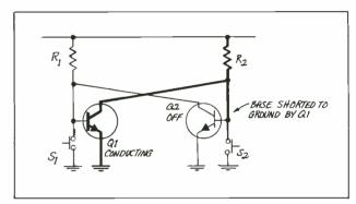
Fig. 1. Simple flip-flop circuit.
