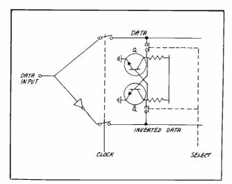
Fig. 6. Flip connected to data and inverted data.
