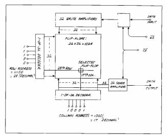
Fig. 11. A 1024 bit RAM in 32  $\times$  32 array.
