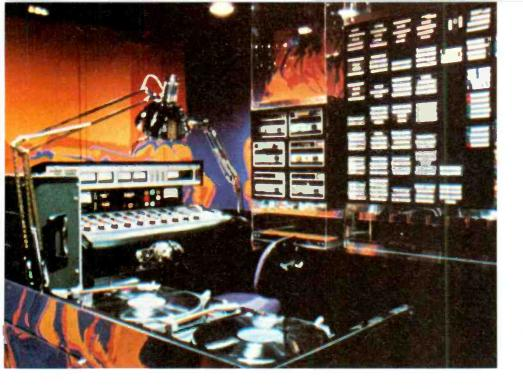
One of the three "on the air" control rooms of the new WQXI AM/FM studios. The equipment consists of custom modified Sparta console with six ITC cartridge reproducers in a suspended frame. Part of the cartridge storage can be seen at right. All consoles are "stand-up" height with everything at the announcer's fingertips.
