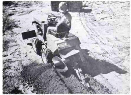
18-HP Model J20 4 wheel drive, with three speed forward plus reverse transmission
