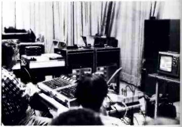
Photos show Mark Schubin, consultant to Lincoln Center before the audio control rack and two Sony audio mix consoles (one for the orchestra, the other production). Recorders are Ampex (for audio) and Sony (video cassette). Stereo channels were located above the video signal (5.8 MHz, L, and 6.6 MHz, R). Subcarriers were set at 0.1V p-p; diplexer was made by Leaming Industries.
