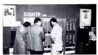
(Above) Schafer 903E full-automation system, introduced at NAB in Chicago, has extended memory for three full days of automatic programming. System shown has six Audiofiles, each holding 48 carts all available for automatic play.
