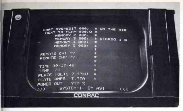
Mitor displays current status of cartridge handling system, including "next to play." Souncer can make changes if needed by simple "edit" process.
