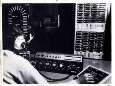
IGM's MARC VII ("manual assist remote control") allows DJ to pre-sequence up to 18 events in advance, interrupt sequence for talk or changes at any time; CRT screen constantly shows event on air, up-coming events.
