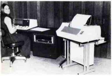
Some stations prefer to own their own computing hardware. Above, a BAT 1500 system from PSI, provides the station with all the computing power this customer needs. As the power and price of minicomputer technology improves the interest in in-house systems increases.
