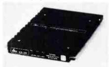
CAT-22 noise reduction card which forms the basis of the Dolby "A" system. Card option allows any 361, M16, or M24 Dolby "A" equipped studio to convert to dbx noise reduction. Cards are supplied in a Halliburton instrument case for ease of carrying. K9-22 cards may be purchased in any quantity at a cost of \$250 per card.
