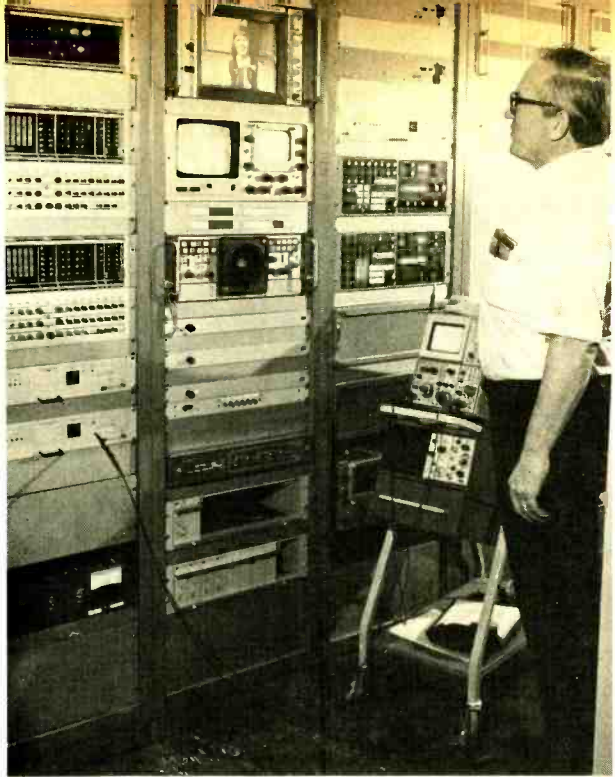
Photo of Vectorscope, picture monitor and Tektronix 1480 R waveform monitor described in opposite column.
