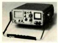
has maximum range of 2000 feet, and can identify impedance changes as small as 0.1 ohm. Model 1503 ranges to 50,000 feet, has 3-foot resolution, and is calibrated in return loss. TEKTRONIX
