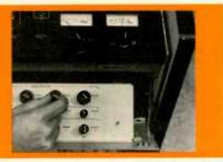
Video head optimizing takes less than a minute on the AVR-2. It's a simple, one-hand operation, as easy as tuning a home hi-fi receiver.
