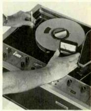
from the cabinet for the most convenient service access you've ever had to a professional one-inch VPR. You can operate the VPR-7900A while the transport is tipped up, and you can observe the effect of adjustments and service operations immediately. That saves time and false moves when making minor repairs.
