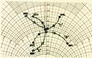
Fig. 1. Plots on Smith Chart show impedance-frequency curves of antenna. Curve A, the original, shows considerable variation at upper and lower sidebands. Curve B is a 45 advance, Curve C, which was chosen, a 45° delay,
