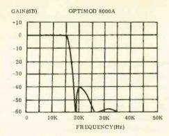
Fig. 10 Frequency response of the new low-pass filter shows the sharp cut-off at 15.3 kHz which removes practically all the harmonics, without causing serious ringing that would raise modulation level significantly above 100%.
