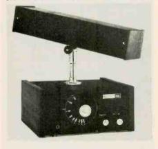
kHz whistle filter is built in. Frequency response is 15 Hz to 10,000 Hz. Sensitivity is 3  $\mu$ V. Companion (separate) ferrite antenna, the DA3, is shielded and directional with FET two-stage amplifier. It can be rotated and tilted to null out unwanted signals. McKAY DYMEK 300
