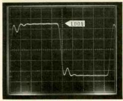
Fig. 8 Response of low-pass filter in new combination unit to 1 kHz square wave shows greatly reduced ringing as compared with other two units; most of ringing is undershoot.
