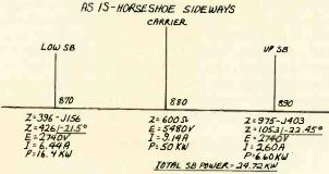
Fig. 2. Calculations show large variation in impedance between upper and lower sidebands of original Curve Fig. 3A (top right). Power and impedance distribution with 600 ohm load, showing even upper and lower sidebands. Fig. 3B (center right). Power and impedance with adjustment to Curve "B" shown on short. Fig. 3C (bottom right). Calculations for Curve chart. Fig. 3C (bottom right). Calculations for Curve 'C", which was produced by a 45° delay network.
