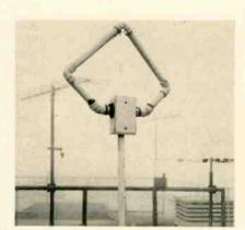
Completed antenna built out of PVC.
