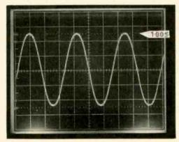
Fig. 9 The response of the filter to a 5.7 kHz square wave shows it reaching precisely 100% modulation, with all harmonics removed.
