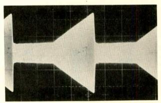
Fig. 5. Ramp waveform, pushing modulation to 135% positive, checks the upper limit of linear positive modulation of transmitter.
