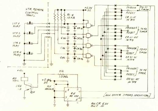
Fig. 1 Blackburn's time and reset system.
