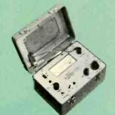
CPB-1 COMMON POINT IMPEDANCE BRIDGE — Monitors common point impedance continuously. Designed for permanent installation.
