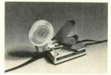
hand-machined dove-tail groove in a hard aluminum block secures the tape. Mount holes and rubber base are provided. \$49.95 + \$1.50 postage & handling. NAGY RESEARCH PRODUCTS 318
