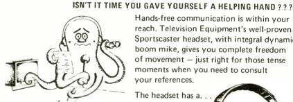
Dynamic Boom Microphone; 400 OHMs, frequency range 50-15,000 Hz, sensitivity 2mV (loaded) for
