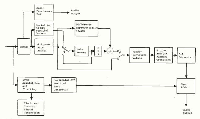
The decoder for the video compression system is essentially the inverse of the encoder operation, providing video output in analog form.
