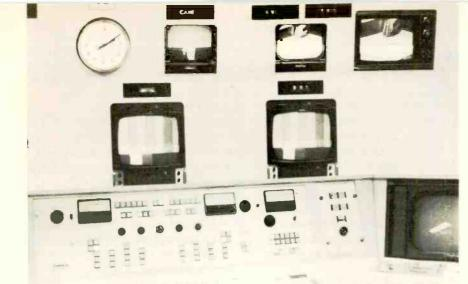
Fig. 1. Monitor bank and section of control console. Right-hand monitor as part of console displays the transmitter signal.
