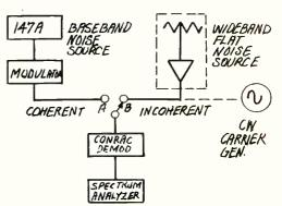
Test set-up used to substantiate the analysis of noise handling in single sideband systems.
