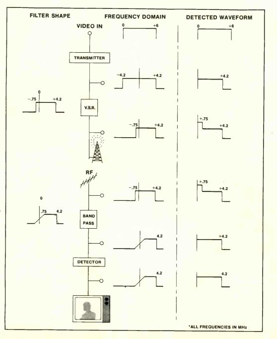
Frequency-domain plot of video signal passband at various points in television transmission system, from video input through detector in receiver.
