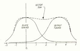
Overall resonance curve for broadband response is indicated above. Arriving at a proper curve requires very careful succession of adjustments, as detailed in story.
