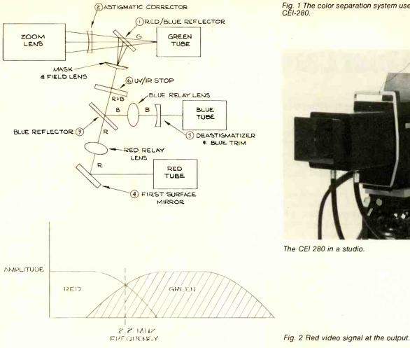
Fig. 1 The color separation system used in the CEI-280.
