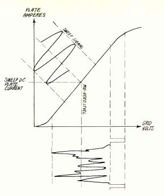
Placement of sweep signal on linear amplifier stage transfer characteristic, for proper accommodation of composite video signal.
