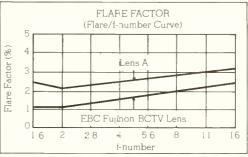
Here again Fujinon lenses have lower flare figures than comparable conventional lenses **6. Spectral Transmission** — Color definition is determined by the degree to which a lens transmits the various wavelengths in the light spectrum. Fujinon's use of rare earth elements in making their optical glass; plus their exclusive Electron Beam Coating make their lenses the ultimate in color transmission.
