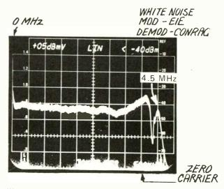
White noise as modulated, then demodulated, showing effects of sideband filtering.
