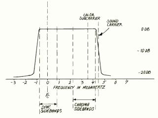
Ideal response curve is shown above. Goal in tuning for maximum power is to obtain as much area as possible under curve between the limits indicated; power at frequencies outside those limits is wasted.
