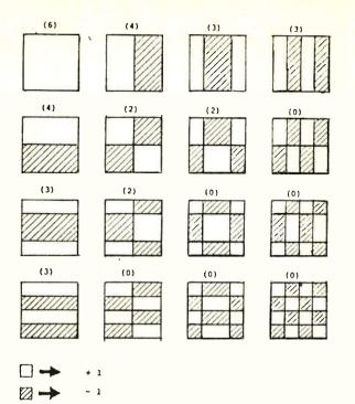
The 16 Hadamard subpictures used in the compressed video system described, which reduces the overall rate to about 8 mb/s.
