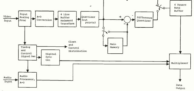
Block diagram of video compression encoder; the A/D converter feeds 8-bit encoded material to Hadamard transformer.
