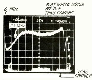
Frequency spectrum of flat white noise at RF, as received , through Conrac demodulator.
