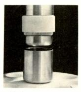
Unusual bullet connector from SWR catches wear particles in cup so they won't contaminate dielectric. Also instead of fingers that wear irrepairably, contact action is confined to a replaceable wristband spring contained by Teflon sleeve. Photo shows lower half of transmission line before it is pushed upward to mate.
