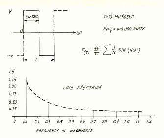
Sync pulse shown upper left is expanded into power series with Fourier formula to right; power carrying information will be in sidebands at odd harmonics of 0.1 MHz carrier, as shown in frequency plot below.
