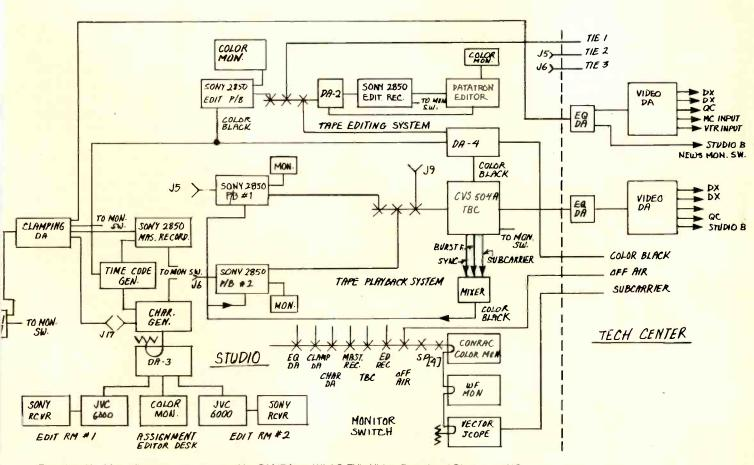
This simplified flow diagram was prepared by BM/E from WLAC-TV's Video Functional Diagram, ENG System. For live airing of tape from vehicle, a patch can be made from J17 to J9.
