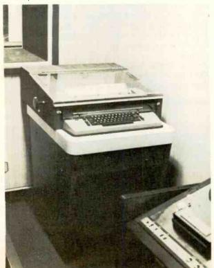
Fig. 5. IBM automatic logging typewriter is to rear of control panel.
