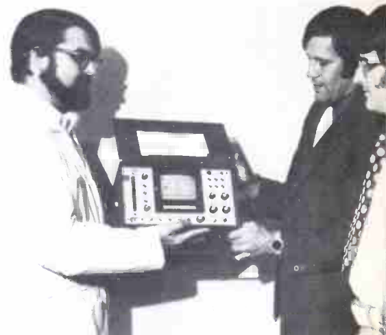
New equipment can expedite system maintenance and analysis. This Jerrold/Texscan visual strength meter can view the sequential response of all carriers instantly.
