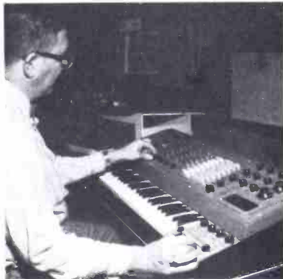
Alfred Mayer of Ionic Industries demonstrates at the keyboard of one of his Putney synthesizers which uses a matrix board with pin inserts for signal routing.
