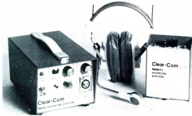
High-intensity interfone can feed a PA system or accept program audio, or both.
