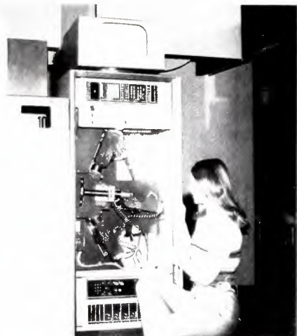
Typical of state-of-the-art telecine equipment, which improves airing of film material by automatic color correction, is new RCA TK-28 system.
