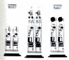
amps in integrated circuits, on card 2½ inches high for 3½-inch file, with PC connector. Others in series are line amplifiers, mike, tape, and phono preamps, summing or mixing amplifiers, etc. FAIRCHILD SOUND EQUIPMENT CORP. 292
