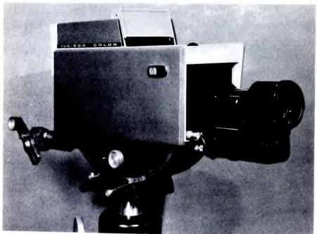
Silicon diode vidicon color camera from IVC
