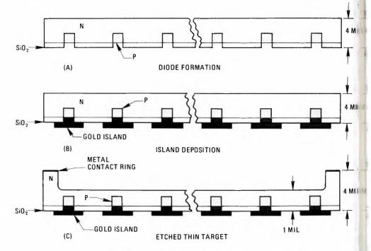
STEPS IN SILICON VIDICON TARGET MANUFACTURE
