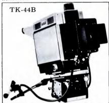
In the NAB "studio of tomorrow" one of the TK-44B's will be shown with a new shot box setup, where a number of shots can be preset automatically. For standard situations, like newscasts, this can automate camera movements—pan, tilt, zoom, as well as raising and lowering the pedestal.
