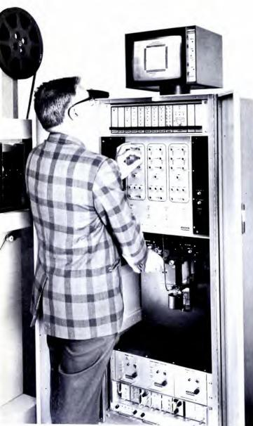
Deflection circuitry is dc controlled and size stability is ensured by 0.1% stable sawtooth generators. Paint, sensitivity, and black level can be controlled remotely.
