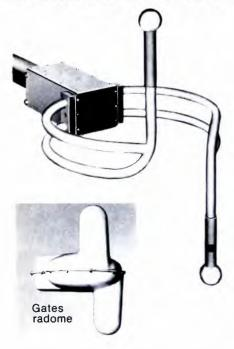
Gates' circularly polarized anterinas combine mechanical ruggedness with transmission reliability. They are constructed of a special brass alloy to withstand corrosion from salt-laden air and industrial gases.
