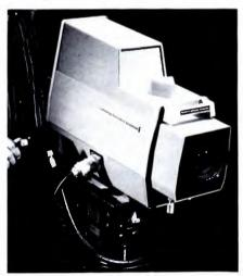
and other engineering functions. A separate panel controlling lens iris, master gain, master black level and paint pots can be mounted near the camera or at a distance. Viewfinder displays a variety of video signals, including a choice of two external sources. \$17,950. COMMERCIAL ELECTRONICS INC. 283
