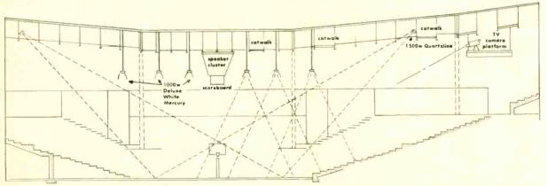
As shown in this cross section of the University of Dayton Arena, three clusters of five Quartzline lamps mounted 60 ft. outside and 60 ft. above each sideline provide additional vertical surface illumination on the court. Close spacing of the fixtures containing mercury lamps over the court assures high and even illumination level on the playing floor. TV camera platform (upper right) suspended from ceiling trusses provides unobstructed non-glaring vantage point.
