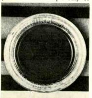
corded signal causes particles to collect into easily-seen patterns. Plastiform tape viewer will aid head alignment, track placement, pulse definition, interblock spacing, drop-out search, and other operations in which a view of the recorded track is useful. Resolution is sharp at the 800 bpi. level and gross flaw detection is possible up to 3200 fci. 3M. 276
