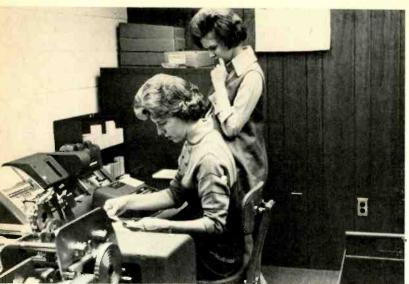
Mary Ann Ratliff and Debra Graybill, WFIR traffic clerks, discuss card preparation for the station's automation system. They are working at the IBM 526 printing summary keypunch; in foreground is the 402 accounting machine. Cards for the system cost \$0.98 per thousand, and WFIR uses about 10,000 per month.
