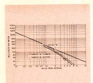
Fig. 2. Illustration of seasonal changes in conductivity. Note the inverse field remains the same, but the conductivity has increased from 5 mmhos/m to 7 mmhos/m.
