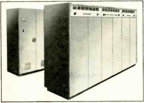
The design is reliability itself. The circuits are solid state design up to the IPA. There are only three tubes in each transmitter. Only two tube types. And the control logic is solid state. That's
