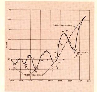
Fig. 5. Plot of transverse radial measurements showing azimuth versus field strength.
