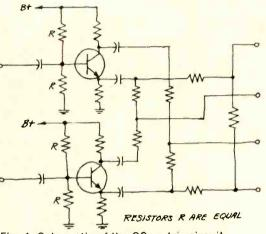
Fig. 4. Schematic of the QS matrix circuit.
