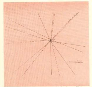
Fig. 1. Example of day-night radials from different towers. In this case, day radials (solid) originated in center of towers number 1, 2, and 6 and night radials from tower number 3.
