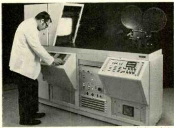
Color video film recorder Model CTR-2 features high-resolution tri-color kinescope, H and V aperture equalizers, comb filter decoder for chrominance/luminance separation, vectorscope, photometer, 10-step gray-scale generator. Camera is 35-mm with f/1.3 lens, driven by closed-loop phase-locked system using air bursts for film advance. Suitable for both negative and reversal color film; scan reversal available. \$75,000. TELEDYNE CAMERA. 290
