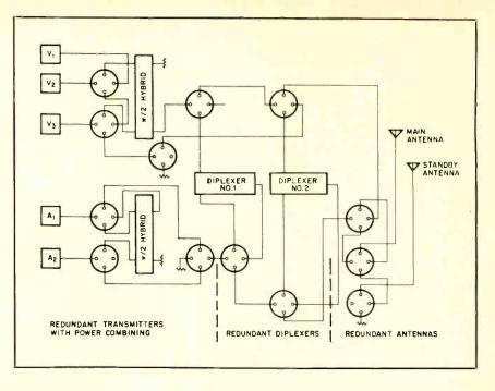
Hypothetical TV broadcast station with remotely controlled rf switching. Depicts redundant transmitters, diplexers and antennas.
