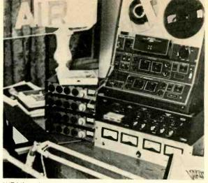
WRNL plays quadrasonic music from 4-channel tapes, such as Project 3 releases, on Sony 4-track tape deck or from RCA 8-track cartridges on Toyo cartridge player. E-V encoder is on bottom of stack. Rerecorded encoded two-channel tape is handled on automation equipment.
