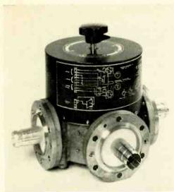
Fig. 1. Motorized coaxial transfer switch  $3\frac{1}{8}$  in. in diameter manufactured by Micro Communications Inc. Switching time is less than  $\frac{1}{2}$  second.
