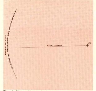
Fig. 4. Illustration of laying out a transverse radial when trying to locate null and lobe positions.
