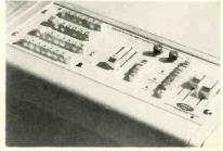
video inputs: seven monochrome comp or non-comp; three color or monochrome composite. Two modes of video matting and keying, front panel selectable automatic sync insertion. CLEVELAND ELECTRONICS. 283
