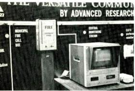
Fire and burglary alarm signals are traced to location by central CRT grid system in the Advanced Research two-way system.
