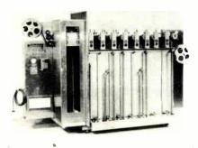
control with thermistor sensor, air squeegee, dry box with dual heat input. FILMLINE CORPORATION. 276
