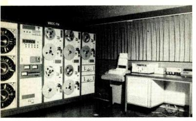
Sono-Mag DP-1 at WROC, Rochester, has five Scully tape decks (right-hand bays), three Carousels (at left end), with control equipment in center including full random access, and storage of 2048 events.
