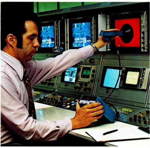
Improve color monitor performance with the TEKTRONIX J16-TV Photometer/Radiometer. Monitor screen color temperatures may be quickly and accurately adjusted or matched, even by unskilled personnel. No individual judgement is required as with visual comparison techniques.
