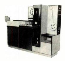
has a processing speed of 24 feet/minute, and a bottom-tendency drive system that minimizes film tension. HOUSTON PHOTO PRODUCTS, INC. 277
