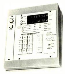
and stop according to a preset program. Sync resolution is 1/300 second and typical search accuracy is 0.2 seconds at 15 ips. AUTOMATED PROCESSES, INC.
