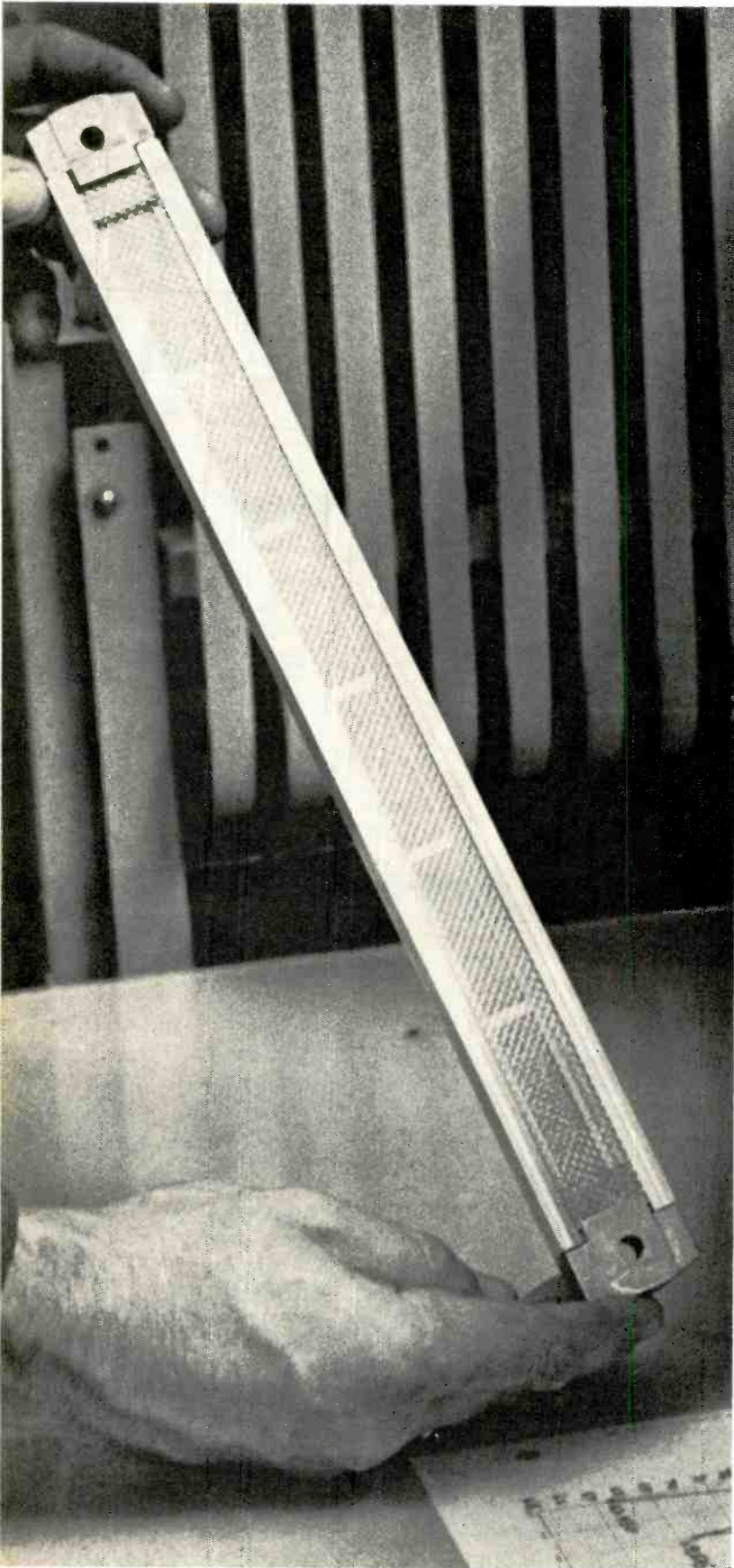
This little bar, containing Microspheres of nuclear isotopes, is a big problem-solver in film-processing equipment.
