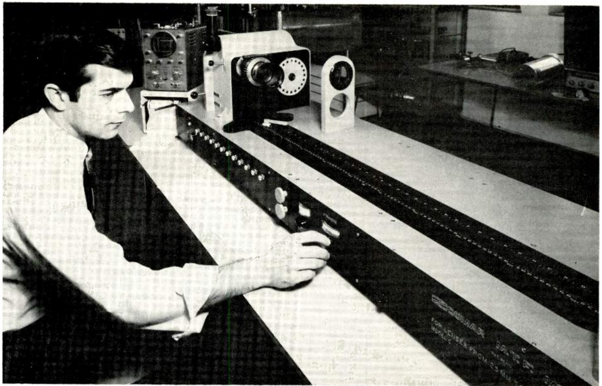
Oscilloscope display indicates accurate focusing on test rig. Chart recorder prints transfer curves automatically.
