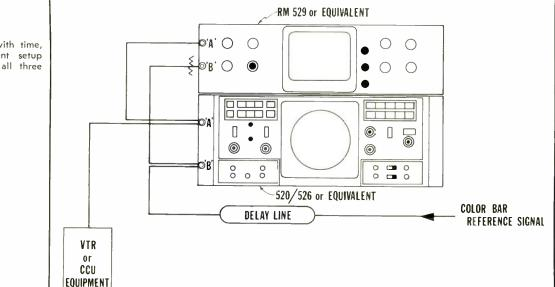
Most economical with time, this test equipment setup can be used for all three basic tests.
