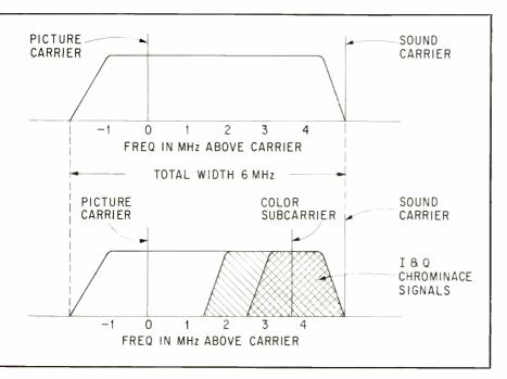
Fig. 2. Frequency spectrum of transmitted TV signals.
