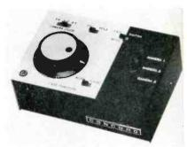
flare fade and superimpose images from a two- or three-camera system. TCP-1 may also be used with any multiple camera system employing an external sync generator. Provision is made for tally light, mic, or other desired connections between operator and cameras. Panel includes video inputs for up to three cameras and a video output for connection to video-tape recorder. Panel measures  $7\frac{1}{2} \times 5\frac{1}{2} \times 3\frac{1}{2}$ , weighs 3 lb, and is priced at \$150.
