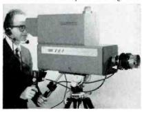
suring 734 × 8 × 2134 in., weighing 35 lb. Solid-state plug-in circuits and operating controls are readily accessible behind flip-down panel for ease of operation and maintenance. Camera control is capable of operating camera through 1000 ft of interconnecting cable. Base price: \$26,500, without viewfinder; \$27,500, viewfinder equipped.
