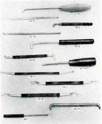
cially designed for adjusting all domestic and foreign type relay spring tension, relay armature back stops, armature arms, etc. Adjuster tips have various shapes and slot openings to accommodate a wide range of relays used in telecommunication and electronic industries.
