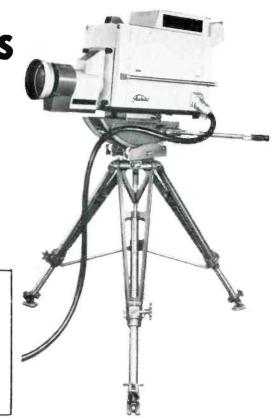
Not hard at all... when it is Toshiba TV broadcast equipment! Besides being compact, the Model IK-37 camera chain provides improved compatibility and sharper pictures with wider grayscale on both types of receiver, color and black-and-white. A 3" Toshiba imageorthicon tube for Y signal and three Toshiba SENSICON tubes for C signal. arranged for easy servicing in this camera head, give signals that are ideal for colorplexing and equal in quality to any straight monochrome signals.
