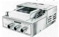
has lighted program indicator, volume, balance and tone controls, positive-select lever and built-in noise filters. Wow and flutter are less than 0.3 percent rms. Output power is 8 W (4 W per channel). Signal-to-noise ratio is better than 35 dB. Frequency response at 3¾ in./s is 100 Hz to 10 kHz. Channel separation, better than 40 dB. Unit operates on 12V, measures  $734 \times 278 \times 878$  in. and weighs 8 lb. Model 3112 is priced at \$59.95.
