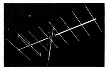
Typical 8-element yagi for Ch. 7-13. This Sitco Model MD-8 offers 13 dB gain, front-to-back ratio of 12.3/1, front-to-side ratio of 7.4/1, is especially designed to withstand severe weather conditions. Sitco makes complete line of cut-to-channel yagis and 2-bay and quad arrays.
