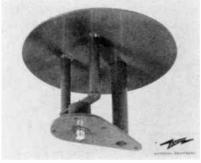
hole. Operating in the 158 to 168 mHz frequency range, the unity gain folded monopole provides a horizontal pattern within 1/2 db of omnidirectional, VSWR is 1.5; impedance is 50 ohms. Price is \$40.
