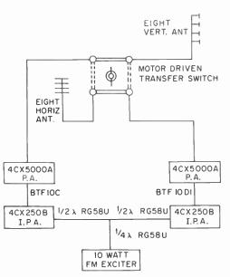
Fig. 1. Block diagram of antenna transfer switch and exciter-IPA connections.
