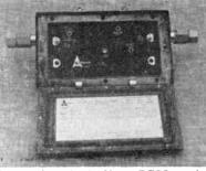
the series, including PSM mainline, PSMB mainline-bridger, PSA mainline with AGC, PSB bridger and PSE extender. PSM features 28 db maximum gain; operating gain is 22 db. Maximum noise figure is 17 db; gain control is 3 db. Housing can be mounted vertically or horizontally with double strand clamp and will accept .750, .500, and .412 cable. Operates within 20-36v AC.
