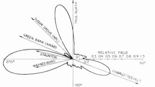
Fig. 4. Horizontal plane radiation pattern designed for Channel 64 (WVIR-TV) Charlottesville, Va.
