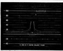
Fig. 1. The Tektronix sine<sup>3</sup> K-factor graticule. Two sweep speeds are provided on these waveform monitors so that this graticule can be used for 0.125 μg T-pulse testing on such applications as studio and network transmission lines, and for 0.250 μs 2T-pulse testing on such applications as video tape recorders and transmitters.
