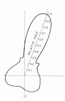
Fig. 6. Horizontal plane radiation pattern designed for proposed Asbury Park, N.J. UHF station.
