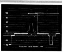
Fig.2. Display of a sine? T-pulse and bar. Waveform shows the following: the horizontal sync pulse on the -40 IEEE unit ine, the backporch on the O-level line, the 10% offset or bas+ for the pulse and bar, and the sine? or T-pulse on the -10 IEEE unit line, and the bar on the -100 IEEE unit line.
