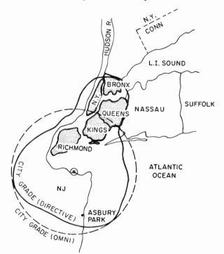
Fig. 7. City grade coverage of Asbury Park station, showing a comparison of directional and omnidirectional disc-rod antenna.
