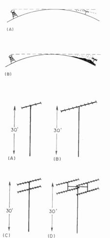
Fig. 1. Over an essentially flat transmitter-to-receiver site path (a), signal level usually can be increased by raising antenna height; 400' to 500' towers are not unusual in some locations. With a naturally elevated receiving site (b) actual tower height seldom has any bearing on antenna output.
