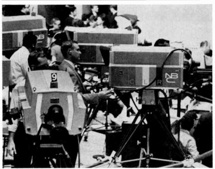
An election night scene at NBC's Studio 8-H in New York. Five TK-43 cameras (only 4 visible) were used in the ballot report, the first time so many of the new RCA color cameras had been used in a single origination. Two will be installed in NBC's "instant news" studio in New York; the other three will be assigned to other studios.
