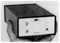
ard receivers. All units are selfcontained, measure  $2\frac{1}{2}''$  high,  $4\frac{3}{4}$ " wide, 8" deep, and can be placed on a shelf or mounted vertically or upside down; a 3unit rack-mount panel is available. Lowband modulator is priced at \$170.
