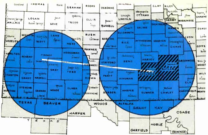
Relative Grade B coverage of 316-kw KAKE-TV Wichita and 87-kw Channel 13 satellite KUP-K Garden City, Kan. The satellite uses a 10-kw transmitter which feeds a 12-bay superturnstile antenna mounted atop an 800' tower. A 6-hop microwave system is used to relay the parent signal.
