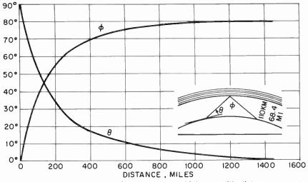
Fig. 1. Two sky-wave propagation parameters which vary with distance.  $\phi = \angle$  of incidence at reflecting layer.  $\theta = \angle$  above horizon at which radiation occurs.
