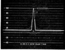
Fig. 3. Display of an undistorted 0.125  $\mu$ s sine<sup>2</sup> pulse at 0.125 H/cm magnified 25X. A T-pulse with its base on the +10 IEEE unit line will reach the -100 IEEE unit line if the video system has 6.7 MHz equivalent bandwidth. At 4 MHz, pulse height will be reduced by 18%.
