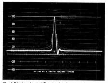
Fig. 4. Display of a sime<sup>2</sup> T-pulse showing some phase distortion. Phase distortion will appear as aberration:, on the leading or trailing edges of the T or 2T-pulse. The K-factor sy::tem relates the amplituee of ringing vs the displacement of the ring from the transient in terms of picture degradation.
