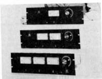
to +40 dbm in 2 db steps, plus a reference setting of 0 dbm (1 mw across 600 ohms) and off. Circuit is designed to bridge 600ohm line.
