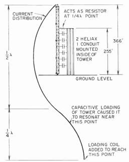
Fig. 2. The presence of the FM transmissions lines and power conduit acted as a capacitor, making AM antenna act as a capacitive reactance.
